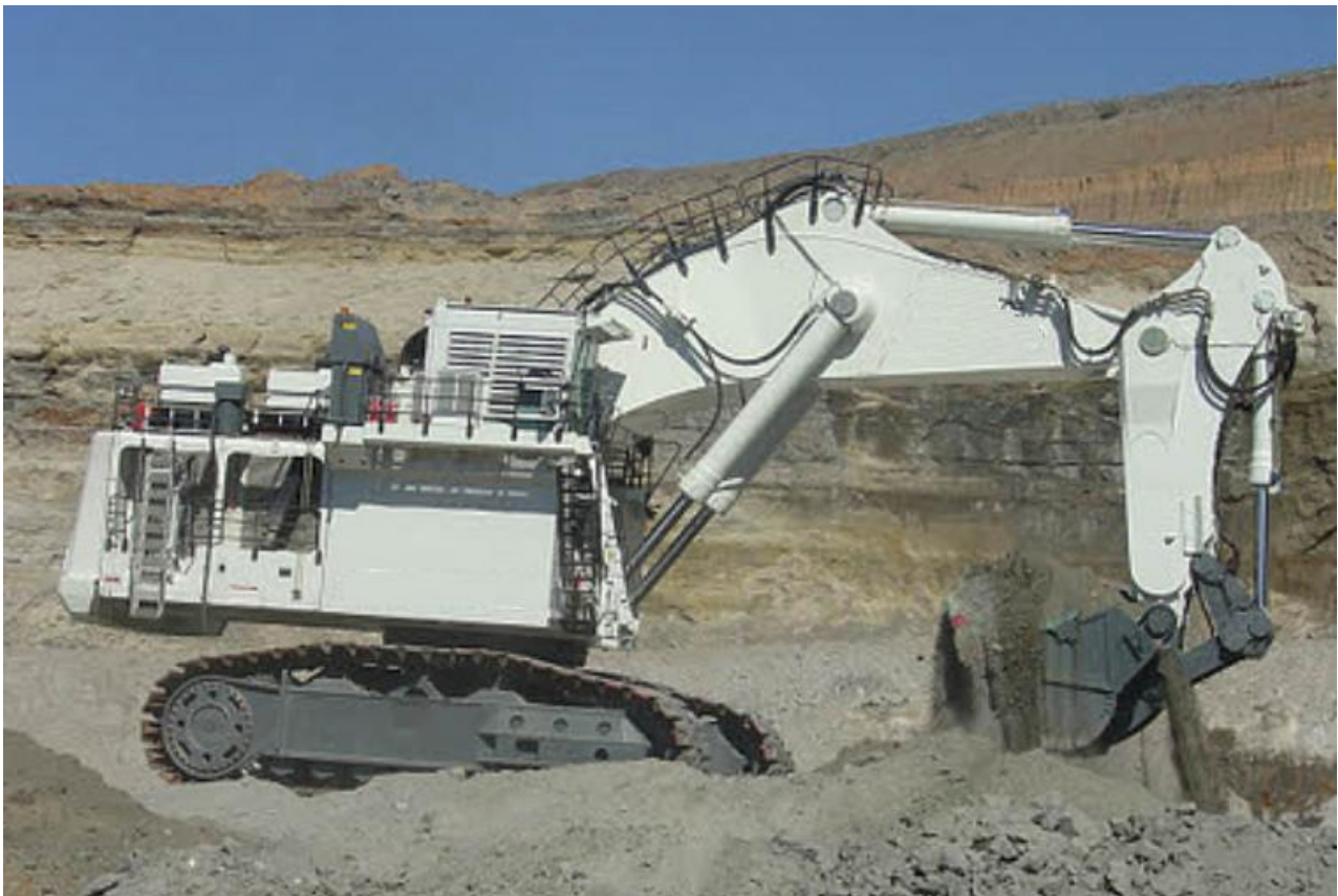
Figure 17. Hydraulic Excavator Set Up as Backhoe
