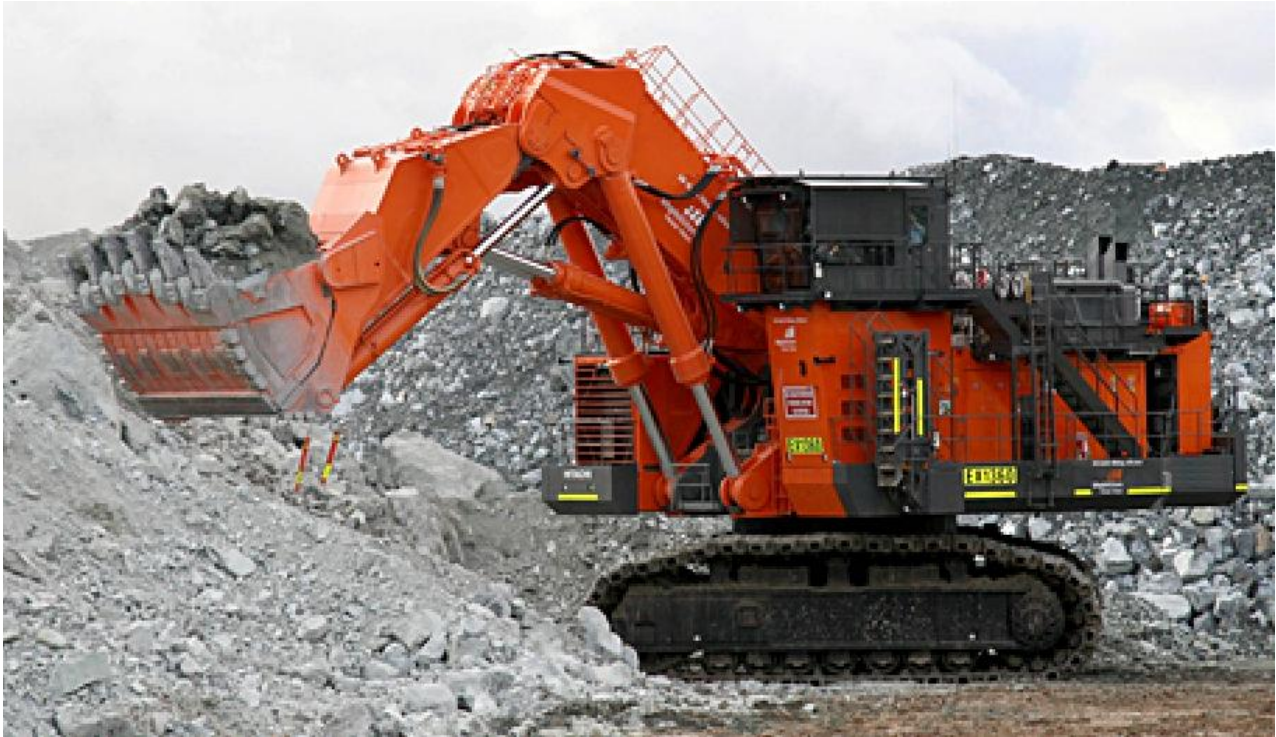
Figure 16. Hydraulic Excavator Set Up as Face Shovel
