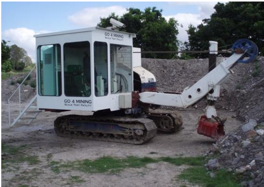
Figure 1: GO4 mining 1:7 scale dragline convertible into a UDD or conventional dragline
